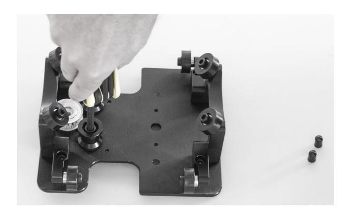
Remove and dis-guard the caps that hold the idler assembly together and secure the two idler pulleys onto the bottom of the cart.
