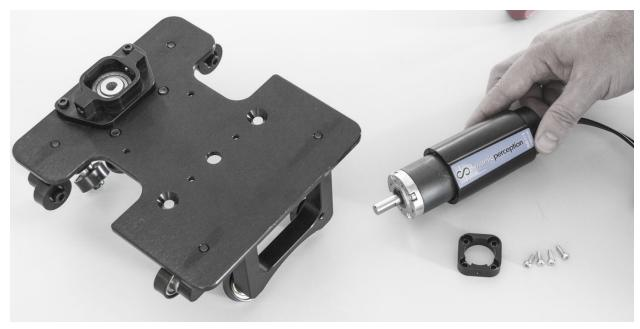
Locate the motor, snap motor mount and 4 mount screws
