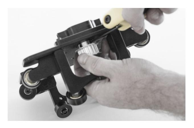
Firmly secure the two lock screws locking the pulley onto the shaft
