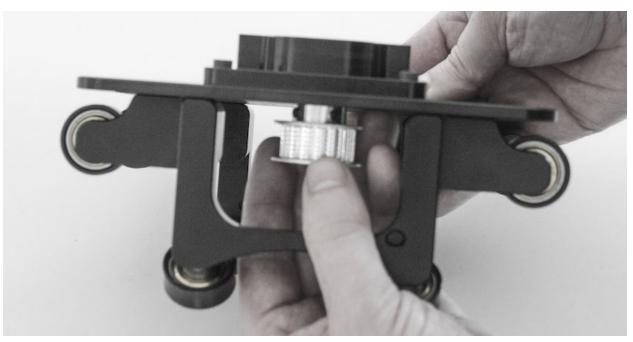
Line the top of the drive pulley with the bottom of the plate
