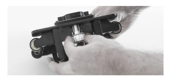
Loosen the drive pulley lock screws and slide onto shaft with lock screws up
