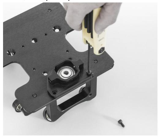
Line up shaft with the largest hole and secure using the mount screws
