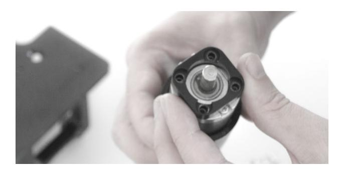
Line the motor mount holes up with the 4 taps on the face of the motor
