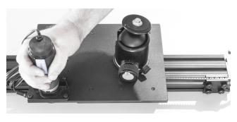
To remount the motor; line the flat part of the motor shaft with the flat part of the inner shaft, rotate the motor to mate with the motor mount and then firmly press the motor in place. It should 'snap' into place. The slider is now ready for motorized use.
