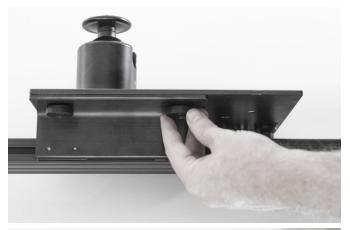
Now re-tighten the knobs to secure the cart onto the rail, the tightness of these knobs can be adjusted to get varying slider pressure on the rail.
