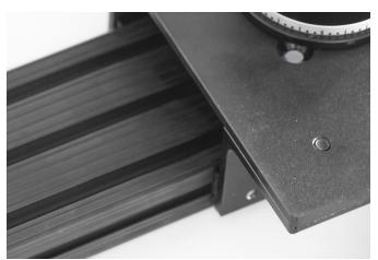
The slider pads should lock into the side slots, the Zero system can ride upside down once the cart is secured onto the rail.
