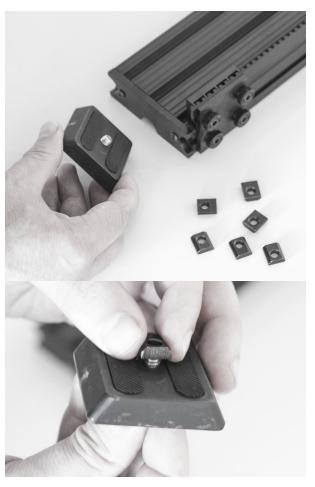
To mount tripods or other supports to the rail use any standard quick release plate. Locate the square 'T-nuts' with 1/4-20 threads (Note: we include extras in case of loss).
