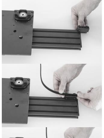
Locate one of the belt clip assemblies (square with 4 small thumbscrews), loosen all four of the thumbscrews on the belt clips to prepare them for mounting. Slide the lower part of the clip into the side slot of the rail with the 'toothed clip' facing up on the same side of the rail as the motor mount.
