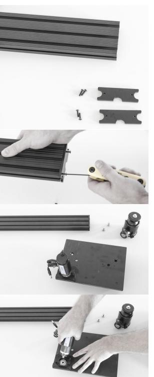
Start by locating the end caps and mounting screws, if you purchased a rail from Dynamic Perception the blue inserts will be pre-installed in the ends of the rail, if you have picked up a #1030 rail from a different source we provide 4 extra inserts, simply pound them into the mount holes at the end of the rail with a hammer (don't be afraid to 'smash' the inserts in place)
