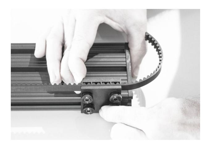
Using one hand pull all the slack out of the belt so it's taught. With the other hand secure the bottom two thumb knobs. The belt is now fully connected, double check that there are no twists and that it's fully meshed with the pulley system. With the motor still out of the system the cart should slide with the belt feeding through the pulley system relatively easily.
