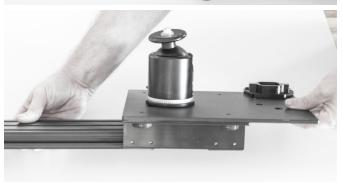
Line the slider pads up with the slots on the sides of the rail, the side cuts in the end caps allow the slider pads to pass through the ends. Carefully slide the cart onto the rail, if you have trouble you can continue to loosen the mount knobs or completely remove one of the slider mounts and re-install once the cart slider pads are lined up with the rail side slots.
