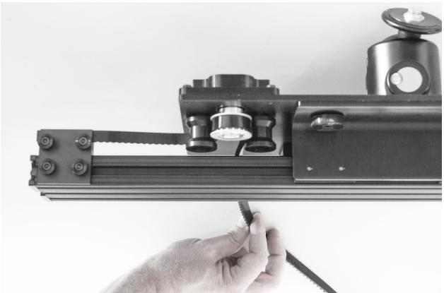
Loop the belt around the outside of the toothed drive pulley and thread it back between the drive pulley and idler pulley.
