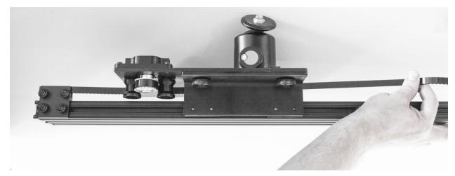
Thread the belt under the center of the cart between the two slider mount uprights.
