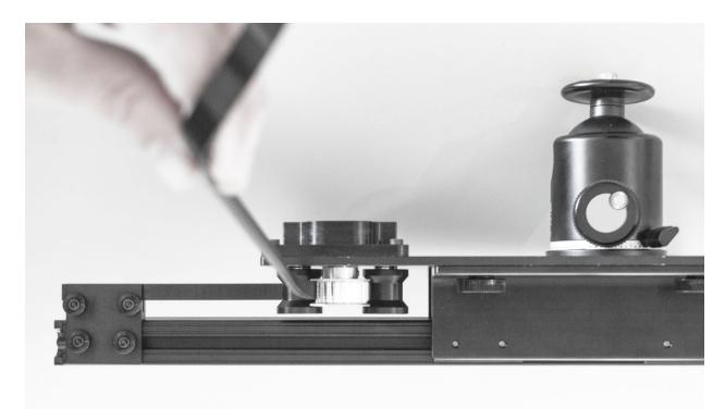
Thread the belt around the first idler from the center of the rail and then between the idler and drive pulley.
