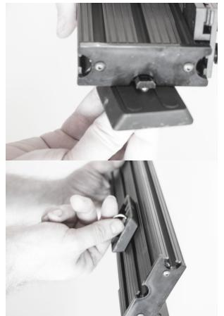
With the T-nut partially threaded slide it into the bottom center slot on the rail.
