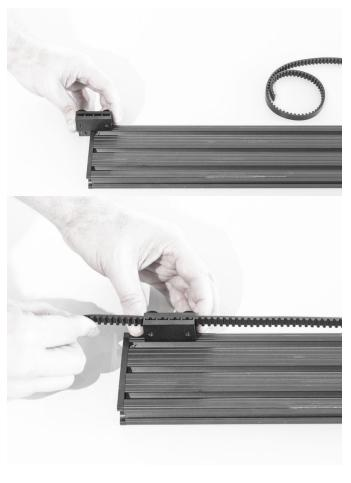
Locate the second belt clip assembly and again loosen all four thumb screws in preparation for mounting, slide the lower clip into the side slot of the rail on the same side as the motor mount and other belt clip.
